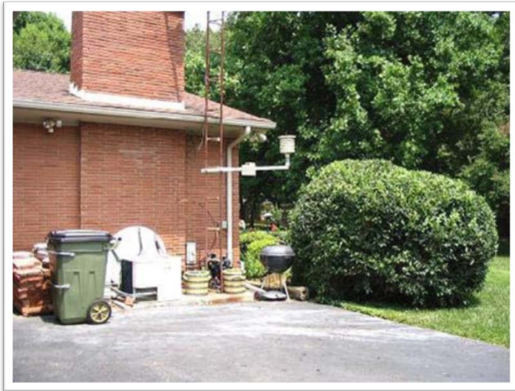
USHCN weather station at Hopkinsville, KY (Pielke et al., 2006). The station is sited too close to a building, too close to a large area of tarmac, and directly above a barbecue.
